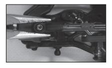
It is important that the turnbuckle eyelets move freely once snapped on to the ballstud. If the fit is too tight, the car handling will be inconsistent. To check, grab turnbuckle eyelet with fingers and rotate the cup. If there is resistance, lightly squeeze ball cup with needle nose pliers as shown and test again. It is important that the ball cup be snapped onto the ballstud before squeezing with needle nose pliers. Be sure to check and adjust the fit for each ball cup that is installed.
